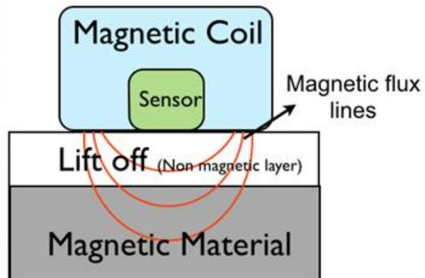
**Figure 2.** 3MA-II equipment and schematic of the experimental setup adopted for the measurements.
