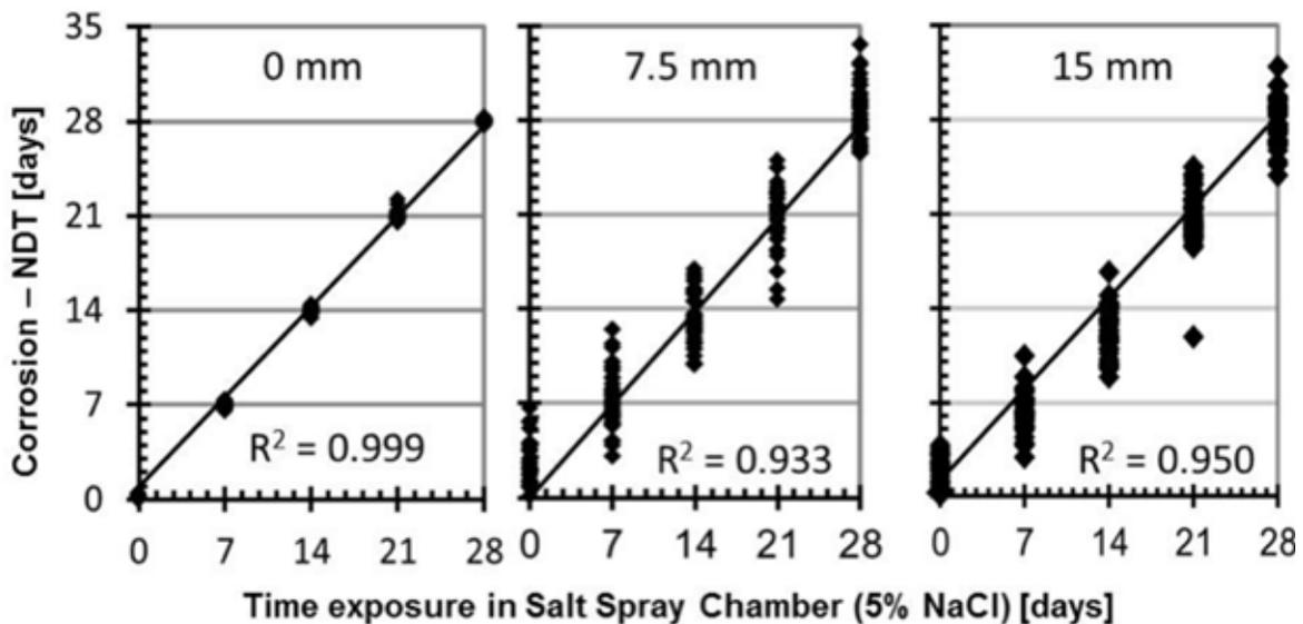
**Figure 4.** Micromagnetic parameters obtained from measurements on samples exposed to varying period lengths: without lift-off (0 mm), and with a 7.5mm-thick or 15mm-thick concrete layer used to impose different lift-offs.
