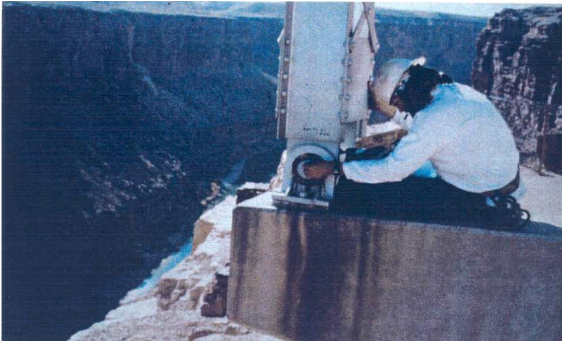
Figure 1.1.3c Ultrasonic testing of a bridge pin.
