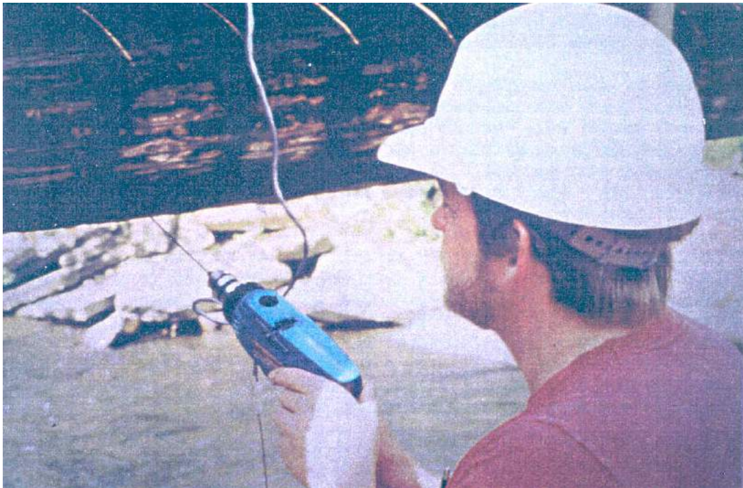
Figure 2.3.3b Drilling of the wood beam in preparation for the shigometer probe.
