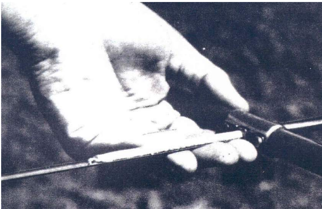
Figure 2.3.4c Wood core removed by an increment borer.
