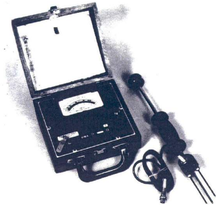
Figure 2.3.3a Typical resistance-type moisture meter.
