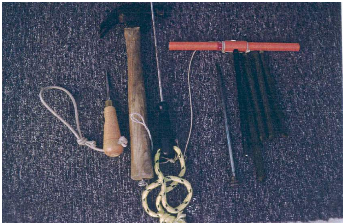
Figure 2.1 Typical tools used for testing wood condition. Left to Right: pick, hammer, probe, coring tool, boring tool and treated wood plugs.
