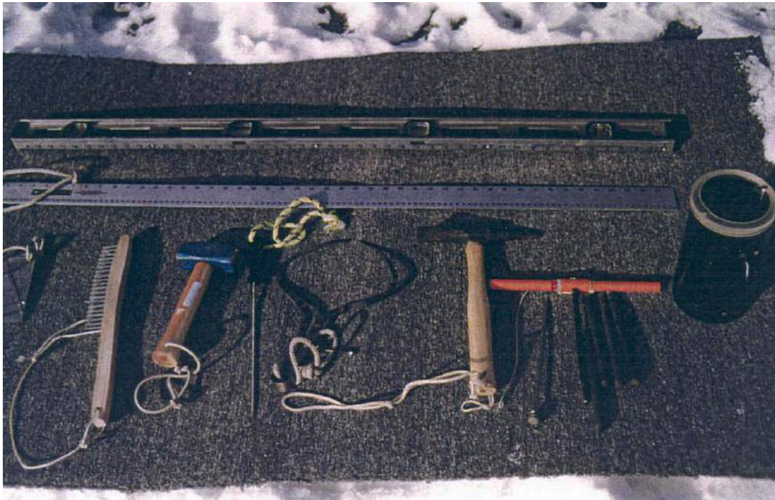
Figure 2.1 Typical Hand Tools for Underwater Inspection
