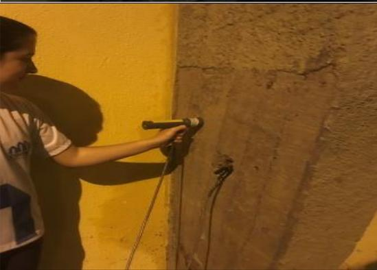
A photograph showing a person using a handheld device (Sensor B) to measure a concrete surface. The device is connected to a cable and is being held against the concrete.                               |
