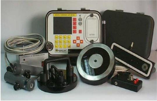
A photograph showing the Gecor 8 equipment kit. It includes a main control unit with a screen and buttons, a carrying case, a circular sensor, a handheld device, and various cables and connectors.      |
