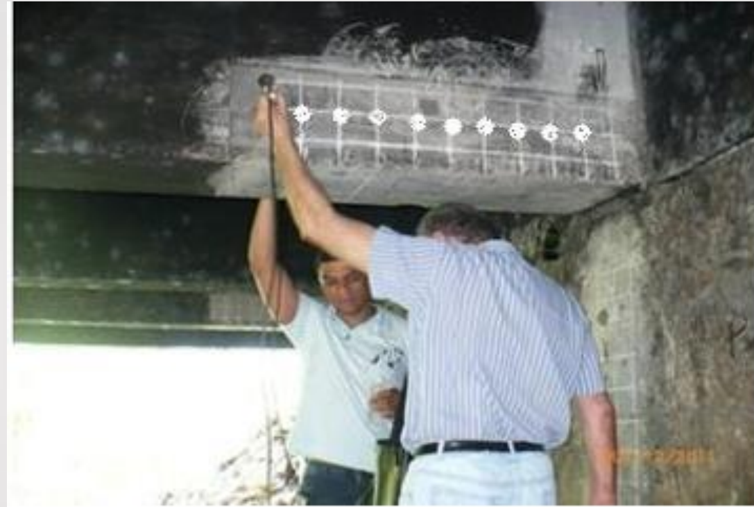
Figure 1. Illustration of the rectangular network used for measurements by impact hammer and ultrasound in a region of maximum stress of a bridge stringer.
